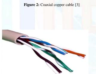
Figure 3: Twisted pair cable [3]
