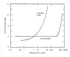
**Figure 4:** Effective attenuation of a 1 km length of coaxial line and glass fiber. The 3 dB bandwidth of the fiber is 500 MHz [8]
